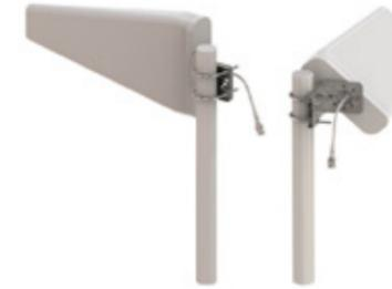
This high performance wide band directional antenna is designed to operate in the 3G/4G/5G bands in Australia. This wideband design eliminates the need to purchase different antennas for each frequency and also means that this model is 5G ready. The brass & aluminium internal components of this antenna are enclosed within a UV-stable white ABS radome for all-weather operation and is supplied with a tilt and swivel mast mount kit.
