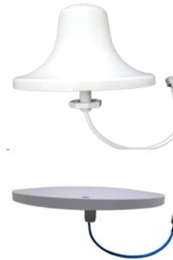
The DAS6938-SOC150-N is a high quality indoor Omni-directional antenna, covering 3G, 4G &5G Cellular bands, 689-960 MHz, 1710-3800 MHz. The DAS3827LP-SOC150-N is a low profile version to reduce the aesthetic impact. These are ceiling mounted antennas and this needs to be considered when planning the installation.
