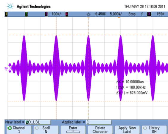
Figure 5 – No modulation (CW) (8 x -20dBm carriers, 100KHz spacing)
