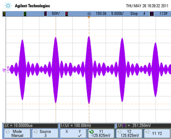
Figure 8 – TETRA modulation (8 x -30dBm carriers, 100kHz spacing)
