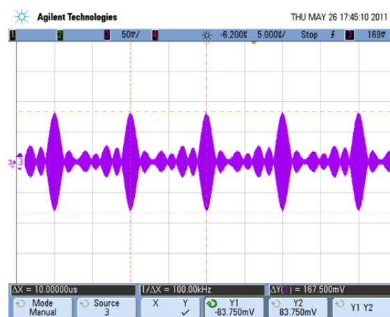
Figure 7 - P25 (phase 1) modulation (8 x -30dBm carriers, 100kHz spacing)
